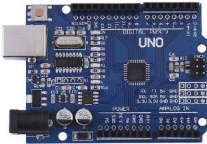
Figure 6: Arduino Uno R3 Pin Layout
